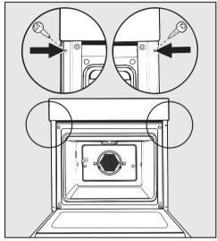
■ Open the oven door and locate the two mounting screw holes in the oven frame. Mark and drill 6 mm pilot holes. Secure the oven to the cabinetry by inserting screws through the frame and into the cabinetry.
